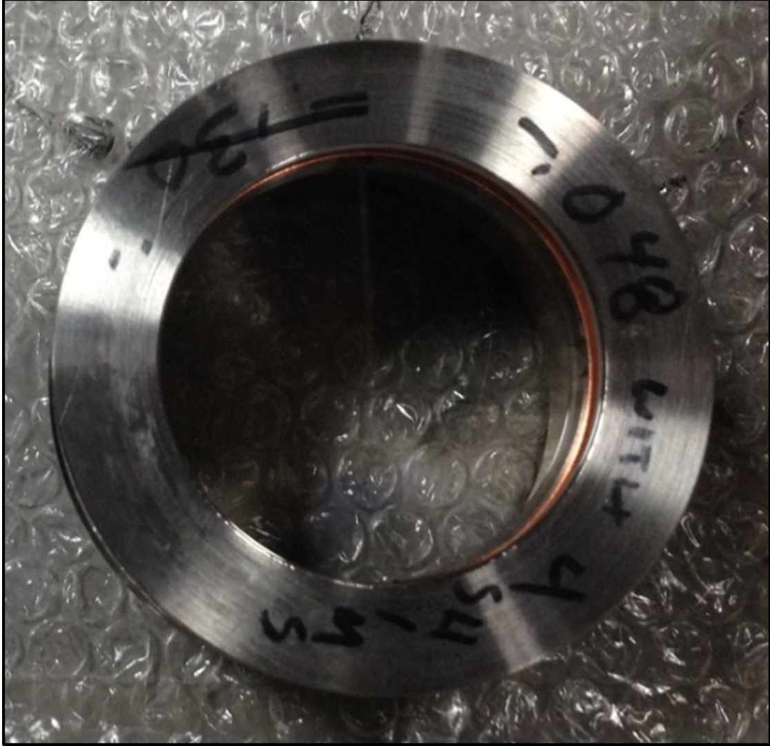
Figure 3-4: The optical piston and Sapphire insert.
